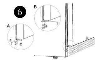
3a. Swap the positions of the hanging Axes (2) and Cap (9) to the opposite side of the door bottom.
