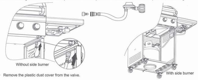
· Screw the regulator coupling onto the tank valve, clockwise, or to the right hand-tighten only.
